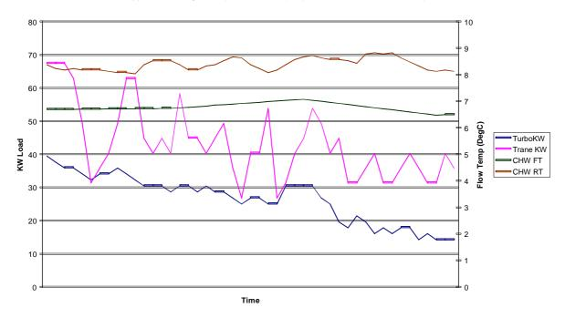
Typical Running: Compressor Load (KW) vs Chilled Water Flow Temps
