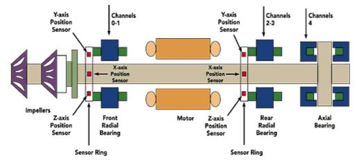
Fig. 2.1 Magnetic Bearing Schematic
